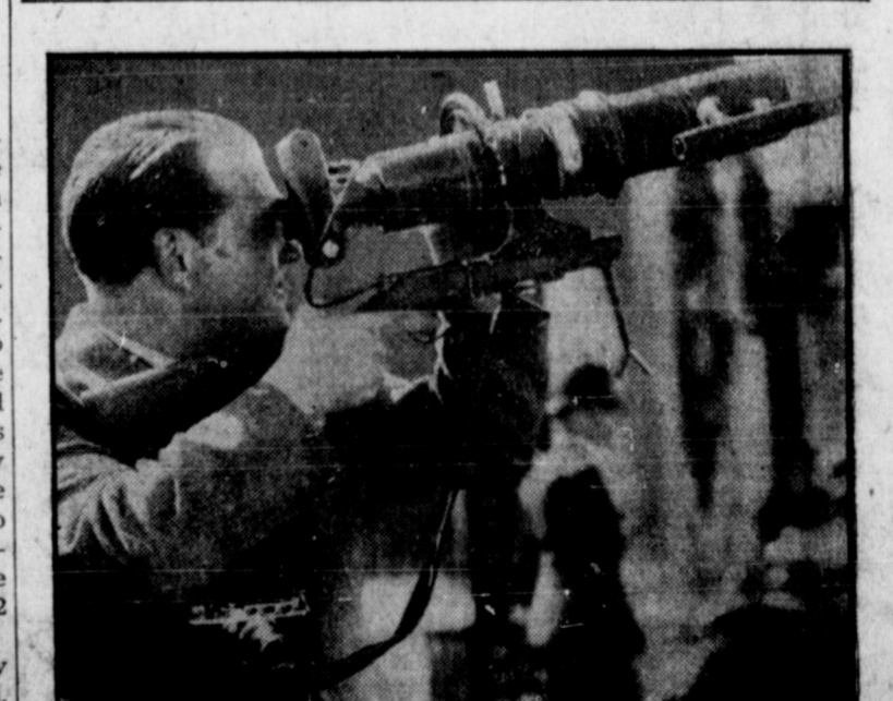
SCENE SHOOTER -Sighting sights with his specially built gun-camera, Werner Wuensch, West Berlin magazine photographer, is able to make rapid-fire takes on 35-millimeter film. The camera is adapted to long shots with a strong lens attached to the end of the "gun barrel."
