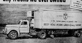
Ford 145-horsepower Model F-7 BIG JOB shows has Gross Combinator Ref rating of 35,000 libs, as a tractor: Gross Vehicle Weight rating of 15,00 h
