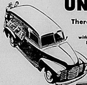
LIGHT DUTY CANOPY EXPRESS Model 3107—116-inch wheelbase, Maximum G.V.W. 4600 lb. Also available in Medium-Duty Model 3807—137-inch wheelbase, Maximum G.V.W. 6700 lb.
