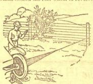
and twist the wires as desired, making a strong cable. With this method he has made cables 150 ft. long.
