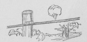
Pumping Air in Cables helps keep your telephone trouble free. Air pressure in the cable holds out moisture should a small leak occur. Reduced pressure as air escapes provides warning of leak so it can be repaired before it affects
