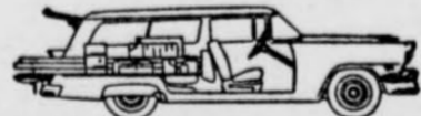
With "Stowaway" seat hidden in floor, you have almost 8 feet of cargo room from front seat to end of tailgate.
