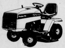
•18 HP Kohler Magnum engine w/oil filter •44", 3 blade vented mowing deck ·6 forward speeds, 1 reverse speed transaxle
