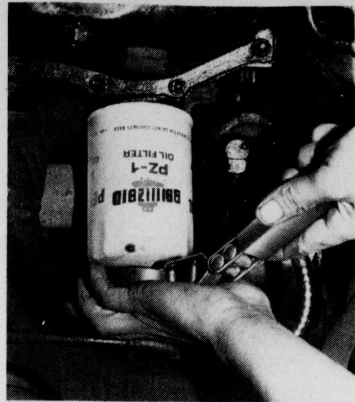
An oil filter wrench, available at any auto supply store, makes changing the filter easy. Merely place a waste pan under the old filter and turn the filter counter-clockwise. Lubricate the new filter gasket with the old oil and spin new filter on in a clockwise direction. Tighten by hand to complete the job.
