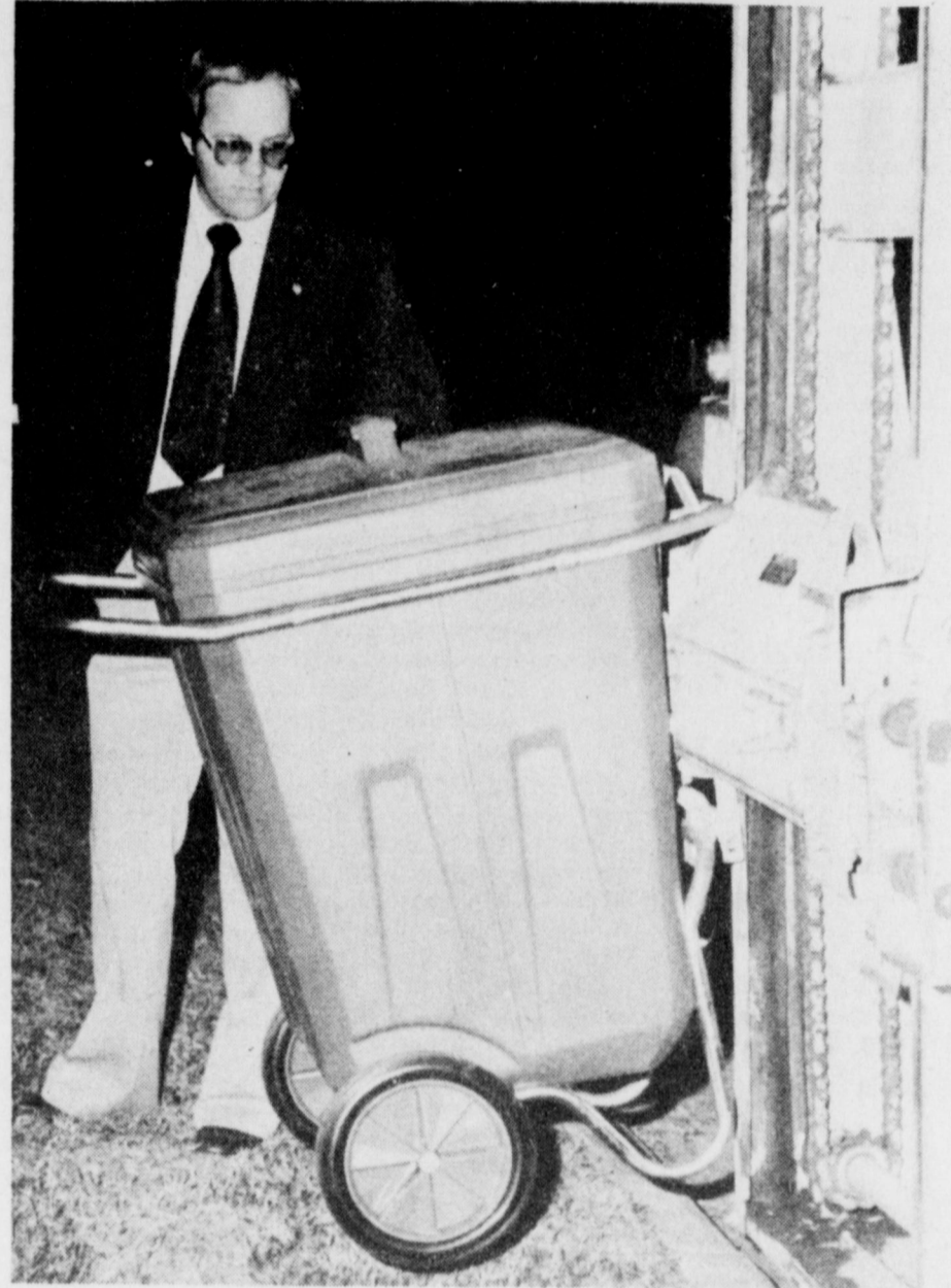
NEW TRASH CONTAINER is demonstrated by City Administrator Steve Morath prior to Monday's meeting of the city council. He shows how the unit is picked up by the trash truck and dumped, without the driver getting out. The unit is proposed for use in homes without alleys where larger units can be utilized.
