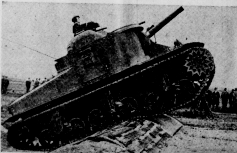
Forerunners of mighty tank fleets soon to roll from production lines roared into the rearward scene in a demonstration at Aberdeen Proving Grounds, Maryland. The tanks can travel more than 25 miles per hour, and mount one cannon and five machine guns. Photo shows M3 medium tank climbing out of a "shell crater" during the tests.
