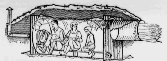
PRE-FAB corrugated steel culvert fallout shelter | radiation exposure of its occupants, is included for three persons can be bought for about \$150, in the "Family Shelter Designs" booklet now plus delivery and installation. The shelter, which at state and local civil defense offices for pubwould cut to 1/500th the amount of outside fallout lic distribution. It is available without charge.
