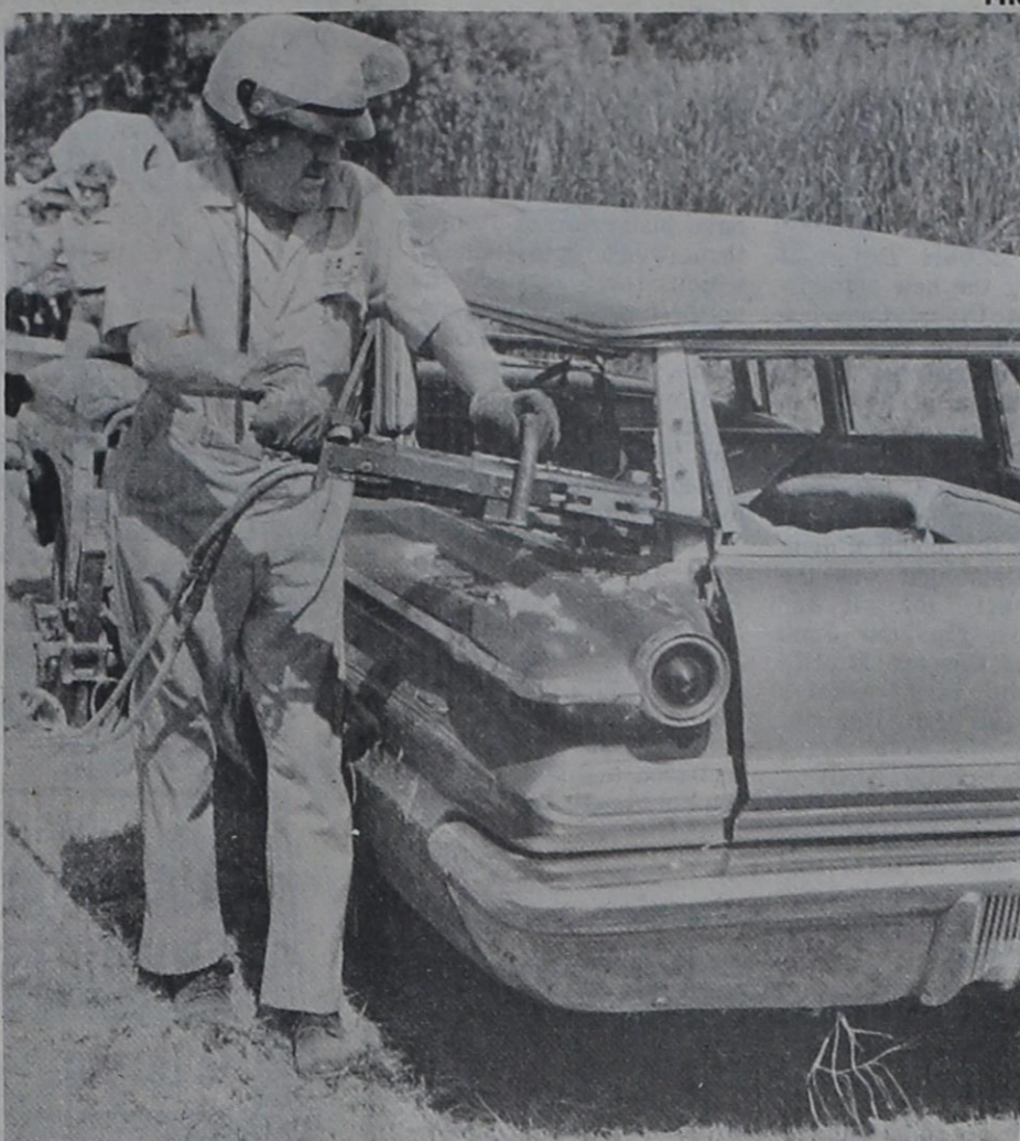
Jim Gill, of Hearst Rescue Tools of New Braunfels, demonstrates the Jaws of Life.
