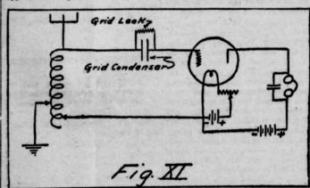
current would flow in the plate cir-cuit and rapidly exhaust the "B" bat-The grid condenser will allow alter-
