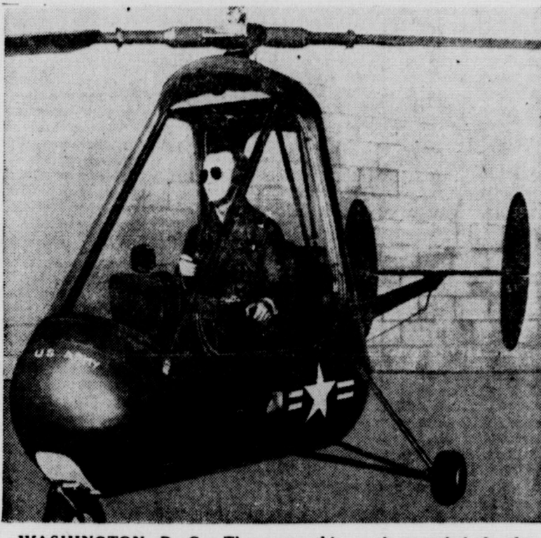
WASHINGTON, D. C.—The army this week revealed development of new-type helicopter, XH-26, which can be dropped by larger planes, unpacked by two men and put in air in 20 minutes. Tiny craft holds two, weighs 300 pounds.
