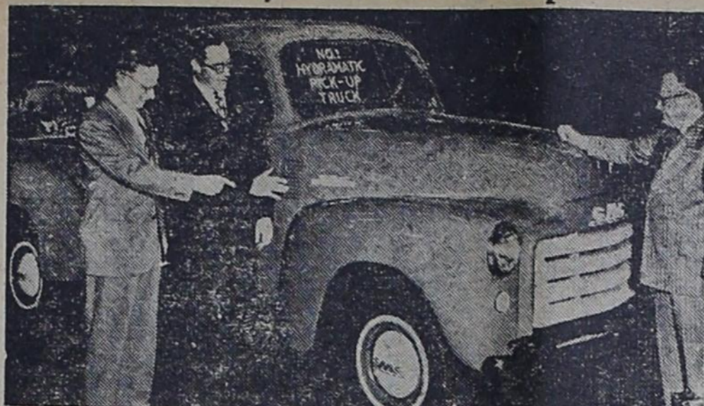
PONTIAC, MICH.—The first GMC Hydra-Matic pickup truck rolls off the assembly line at the GMC Truck plant as three GMC officials point out the "GMC—Hydra-Matic" insignia. Nineteen GMC 1953 light truck models now have the famed Hydra-Matic drive available, plus a new 228 cu. in. engine of 105 horsepower and a compression ratio of 8-to-1. Standard grade fuel is used.
