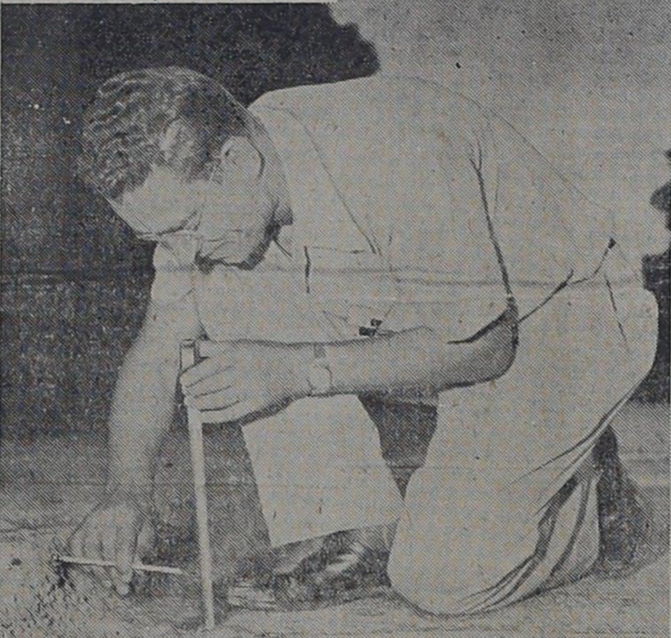
CONCRETE EVIDENCE —Scientific study of how highways crumble under truck loads of varied weight is the six-month test of a 1.1-mile strip of road in Maryland under 11-state sponsorship. U.S. engineer shows how one section sagged three inches under constant use by 11-ton truck in 90 days. Tests will continue through December.
