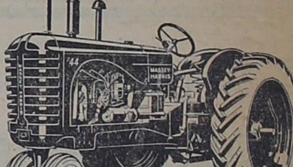
3-4-Plow "44"—260-cubic-inch, 4-cylinder engine, 5 speeds forward.
