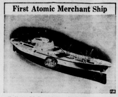
The Nuclear Ship Savannah, the world's first commercial nuclear-powered ship, is a milestone in the history of the Merchant Marine. With an atomic reactor as the source of power, the Savannah can carry 10,000 tons of cargo and 160 passengers and crew 350,000 miles without refueling - equivalent to 14 times around the equator, or 113 Atlantic crossings
