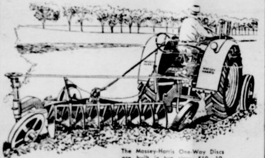
The Massey-Harris One-Way Discs are built in two sizes: 510-10-inch spacing 24" discs, 6, 8 1/2, and 10-foot sizes; 509-9-inch spacing, 24-inch discs, 6- and 8 1/2-foot sizes.
