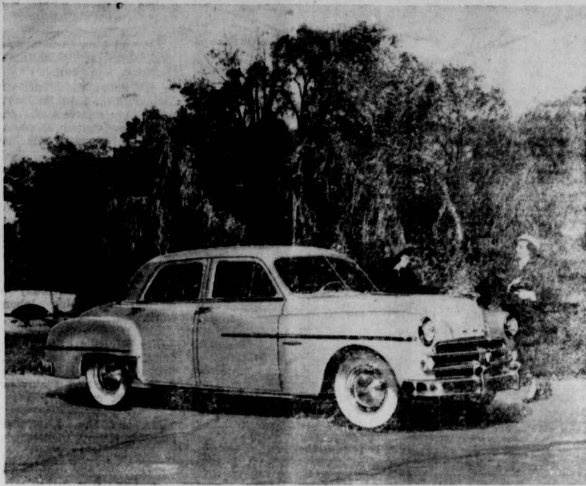
New body lines, larger rear window and fresh front end styling identify the new Dodge Coronet four-door sedan. The new Dodge line consists of ten body styles on two wheelbases. Coronet models, on a 123 1/2-inch wheelbase, are available with Gyro-Matic transmission, which frees the driver from shifting. Fluid Drive is standard equipment on all Dodge cars.
