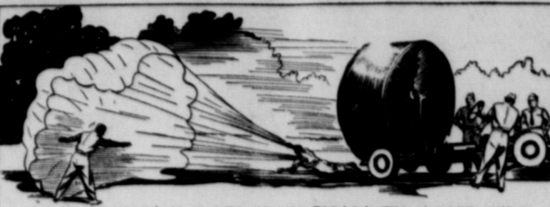
AN AID IN TEACHING PILOTS TO USE PARACHUTES IN STIFF WINDS IS THE AUTOMATIC WINDSTREAM WHICH IS EQUIPPED WITH A PROPELLER THAT ACTS EXACTLY THE SAME ON THE GROUND AS IT DOES IN THE AIR
