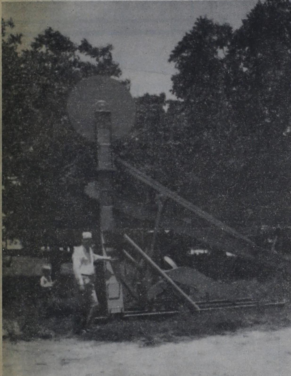
Gaddys Wheel Jack-This is a WA114 Wheel Jack shown by its inventor, Arthur Gaddy. This wheel jack uses 30-40% less energy than Lufkin.
