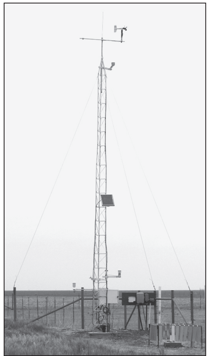
NEW WEATHER STATION —In cooperation with the West Texas Mesonet, the National Weather Service in San Angelo and Rolling Plains Groundwater Conservation District, a weather station has been erected one mile northwest of Haskell to provide continuously updated weather information. The station is connected to the internet and provides updated information every five minutes. The station provides information on temperature, humidity, wind speed and direction, peak wind gusts, rainfall, max and minimum temperatures, frost durations and solar radiation. These readings will be invaluable in weather forecasting and in management of the Seymour Aquifer. The weather data may be accessed anytime at www.mesonet.ttu.edu . The West Texas Mesonet website also has available surface maps and radar loops. Another interesting feature is a meteogram, which is a graphic representation of the weather and its changes in the last 24 hours. The website also provides access to 56 other weather stations in West Texas.
