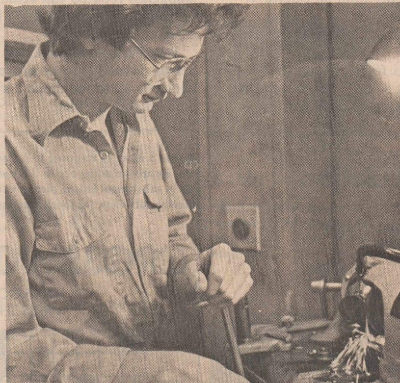
IT'S A GREASY JOB, BUT... — (Above) Scott Groat, Russell Smith and Frank Moreno contribute their efforts to knocking out old cam bearings in a motor in automechanics class, to be replaced by new bearings. (Right) Russell Smith grinds valves to reseal them. Automechanics is one of the vocational education classes offered at WTC observing Vocational Education Week proclaimed by Governor Mark White.
