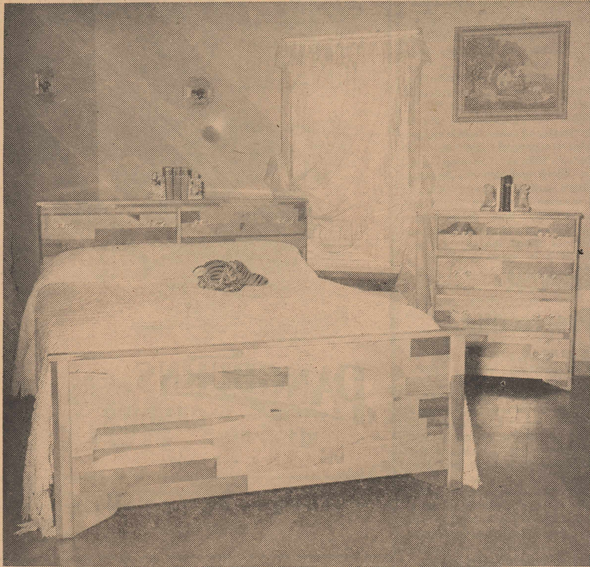
Mr. Adair made the bookcase headboard bed and chest to match out of white pine. He constructed them without nails—they are put together with glue and screws. The pretty wood was shellacked and then varnished for the glossy finish. (STAFF PHOTO)
