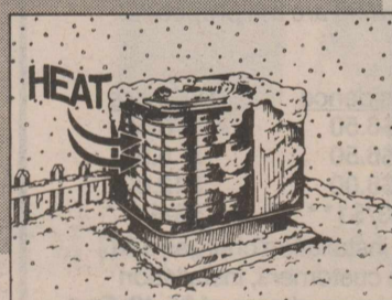
There is heat in the air on the coldest days. The heat pump captures it to warm your home.
