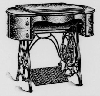
This is an AUTOMATIC LIFT drophead stand with an absolutely positive and easy action accom-plished with mechanism of extreme simplicity. When the table leaf is swung over the sewing, the head of the machine is automatically lifted to place and locked firmly, and when the leaf is closed the head is low-ered into the dust-proof receptacle provided for it. Nothing more per-
