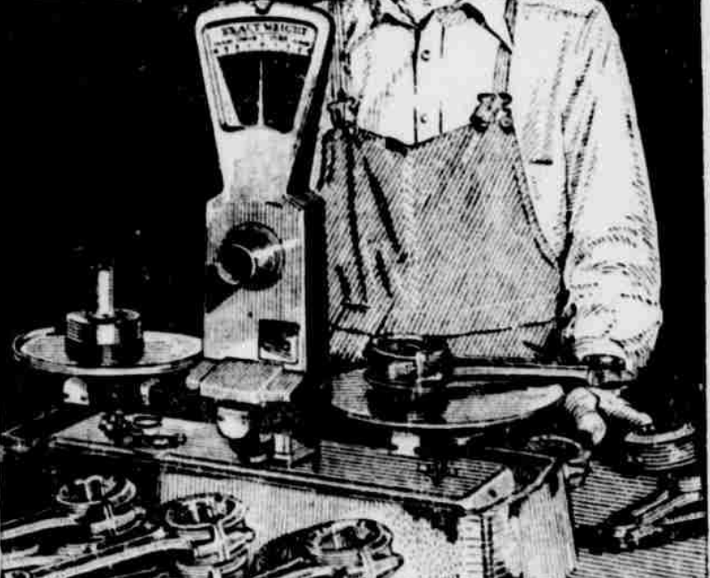
Chevrolet connecting rods are matched in sets of six to within one-quarter ounce, and are individually fitted by hand to the crankshaft. Holes are of babbit metal cast into the rods under heavy air pressure and at 800 degrees Fahrenheit.
