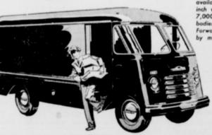
FORWARD-CONTROL CHASSIS Model 3942—137-inch wheelbase Maximum G.V.W. 10,000 lb. Alse available in model 3742-1251/4inch wheelbase, Maximum G.Y.W. 7,000 lb. Package Delivery type bodies suitable for mounting on the forward-Control Chassis are supplied
