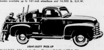
Model 3104-116-inch wheelbase, Maximum G.V.W. 4,600 lb. Othe models available: 3604—1251/4-inch wheelbase, Maximum G.V.W. 5,800 lb; 3804—137-inch wheelbase, Maximum G.V.W. 6,700 lb.
