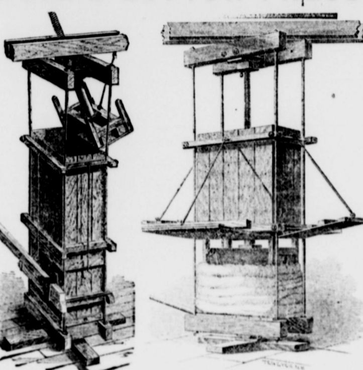
Showing Follower being made for admission of Cotton. Showing Position of Parts when ready for Use.
