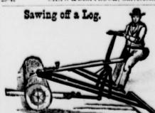
This SAW MACHINE is a wonderful invention. The weight of the man who is sawing does half of the work. It saws logs of any size, and will saw off a 2 foot log in 2 minutes. Circulars free. Address, Wm. GILES, 696 W. 6th St., Cincinnati, Ohlo.
