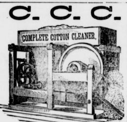
The Complete Cotton Cleaner, a New, Valuable and Moneymaking Machine to every Cotton producer or ginner,-thoroughly removes all Dust, Diet, Sand and light TRASH from cotton before ginning, and improves tha quality of the list from one to four grades.
