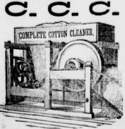
The Complete Cotton Cleaner, a New, Valuable and Moneymaking Machine to every Cotton producer or ginner,-thoroughly removes all Dust, Dirt, Sand and light TRASH from cotton before ginning, and improves the quality of the lint from one to four grades.
