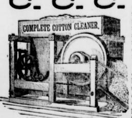
The Complete Cotton Cleaner, a New, Valuable and Moneymaking Machine to every Cetton producer or ginner,-thoroughly removes all Dust, DIRT, SAND and light TRASH from cotton before ginning, and improves the quality of the lint from one to four grades.
