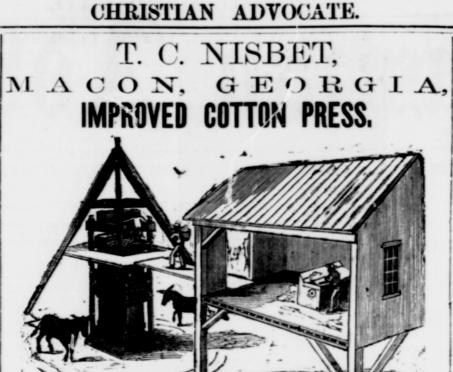
This Press is similar in principle to the old Wood Press. The material of the Screw is Iron. The first cost is less and the workmanship much more perfect than the old Wood Press. C.
