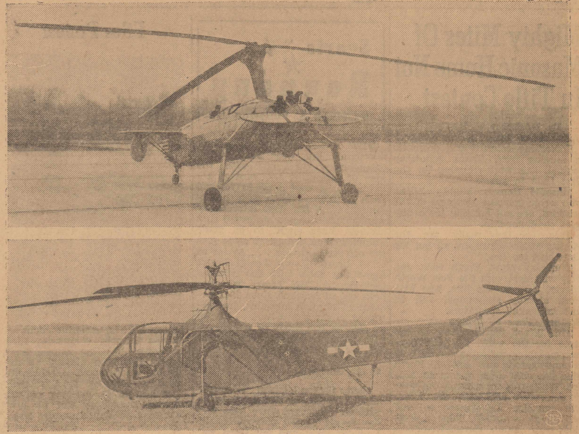
(U. S. Army Air Force Photo From NEA) Main difference between these two windmill-type airplanes is that one has a propeller in front, the other has it on the tail. The autogiro, top, actually a trade name for one type of gyroplane, uses a regular propeller for forward motion and has the large wind-blown rotor instead of a fixed wing for lift. The helicopter's rotor is motor-driven, runs the plane up and down as well as forward or backward. Small rotor in rear keeps the helicopter from spinning around.
