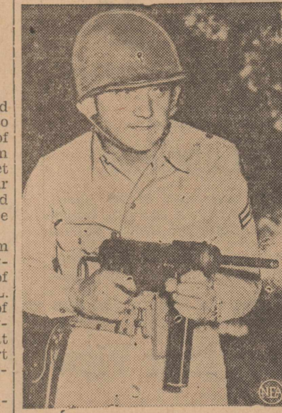
Small but sturdy is the Army's new M-3 sub-machine gun, a .45-caliber weapon weighing less than nine pounds, costing less than $20. (Garand rifle weighs 9 1/4 pounds, costs $85; Thompson sub-machine gun weighs 12 pounds, costs $10.) (Army photo.)
