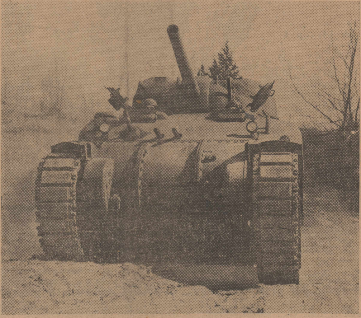
Thundering over a ridge at Ft. Knox, Ky., testing ground comes the Army's new rivetless medium tank complete with 75 mm. gun and a battery of machine guns. The M-4 has an all-cast body and mounts its big gun on revolving turret in center instead of lower down on the right side as on the M-3 tank.
