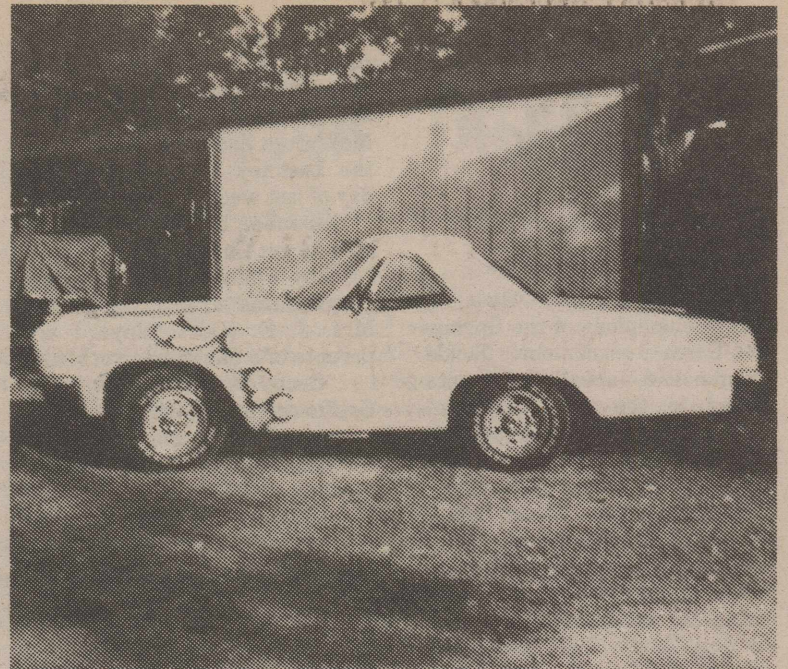
Leon Lavy recently manufactured this car by taking 36 inches out of the middle of a 4-door Chevrolet Impala. The totally unique vehicle now belongs to Lavy's brother.
