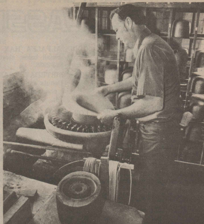
Kenneth Rhyne has been making hats for over 18 years at Roberts Hat Factory in Abilene. Here, he puts a hat through the blocking press where steam heat will set the size and shape of the crown. Rhyne’s shop is one of the leading hat shops in West Texas, and offers a variety of materials, styles and colors to suit the most discriminating buyer. Tx Tourist Agency photo.
