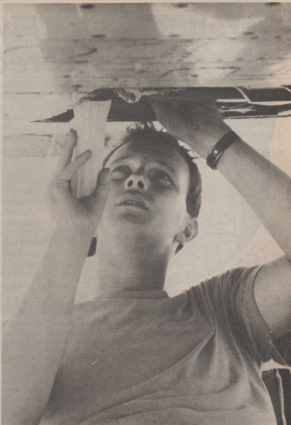
Sgt. Vince Bowling checks flight control rods on a T-38. Sergeant Bowling is assigned to the 64th Organizational Maintenance Squadron. (U.S. Air Force photo by Sgt. Mike Breslin)
