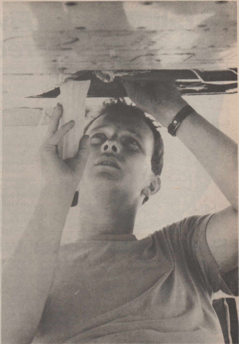
Sgt. Vince Bowling checks flight control rods on a T-38. Sergeant Bowling is assigned to the 64th Organizational Maintenance Squadron. (U.S. Air Force photo by Sgt. Mike Breslin)
