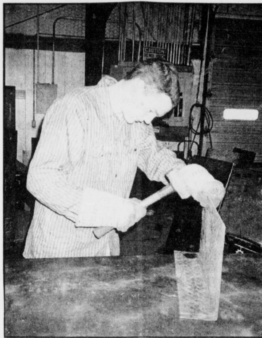
JOSH GRIFFIN -Rivercrest FFA student chips away the bad beads on welded metal.
