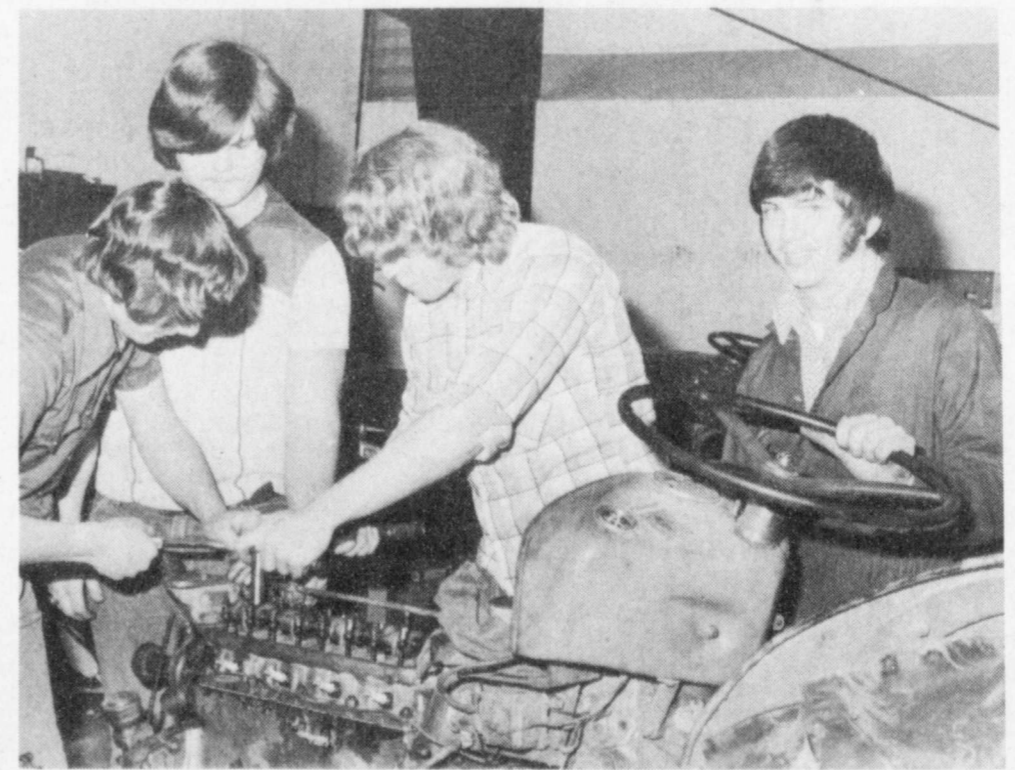
ROCKER ARMS—Joel Hanks, Edward Deaton, Steve Alford and Jeff Baughan adjust the rocker arm assembly on a tractor in the shop at Rivercrest. Tractor mechanics classes rebuild tractors and other farm equipment in an instructional environment. (Staff Photo)
