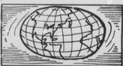
The earth is not perfectly round. Distances measured through the poles are shorter than those at the equator.
