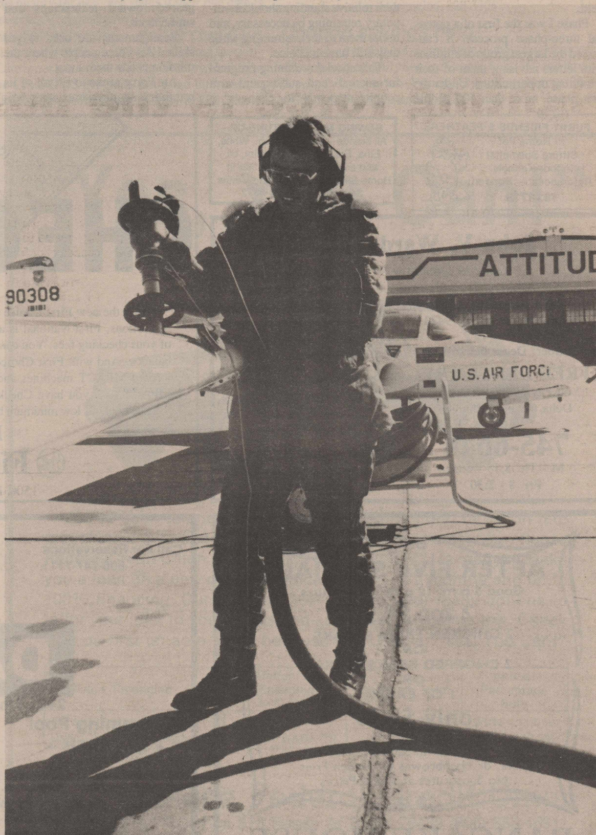
Staff Sergeant Ken Warner, a T-37 crew chief assigned to Cobra Flight, 64th Organizational Maintenance Squadron, refuels a T-37 between flights. The T-37 will hold 326 gallons of fuel. The Maryville, Tenn. native has been assigned to Reese for four years. (USAF Photo)
