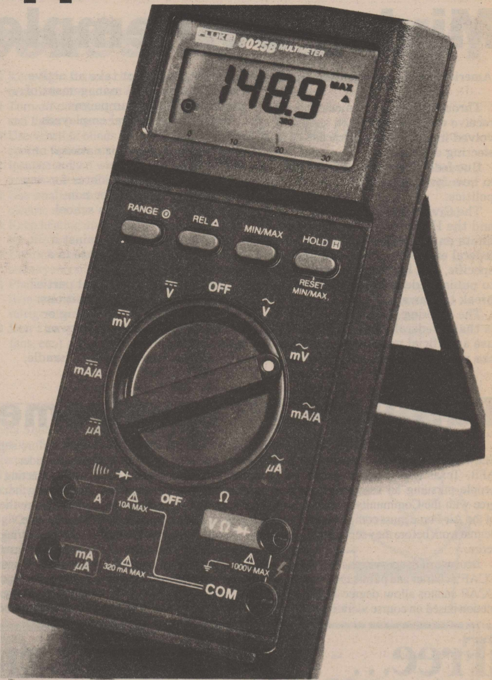
The Air Force's new multimeter can withstand explosions and 35-foot drops and can resist water and chemicals. (Air Force photo)
