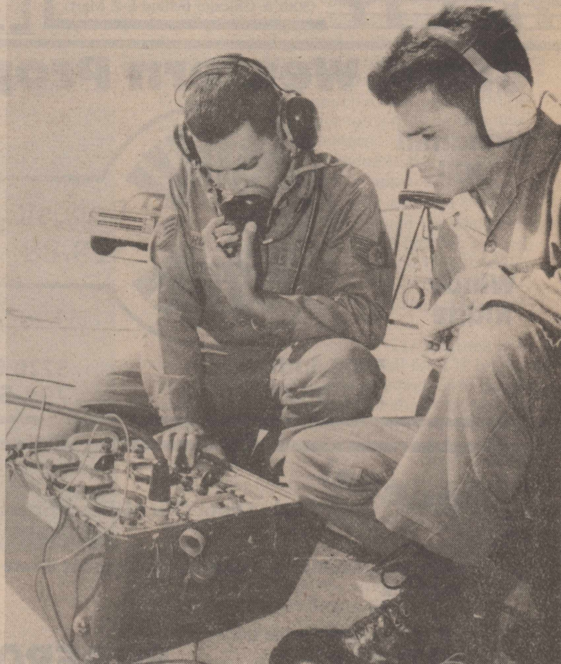
Sgt. Willie Ruiz (left), a day-shift flightline supervisor for the electrics shop, helps Amn. Thomas Garcia trouble shoot a T-38 generator malfunction.
