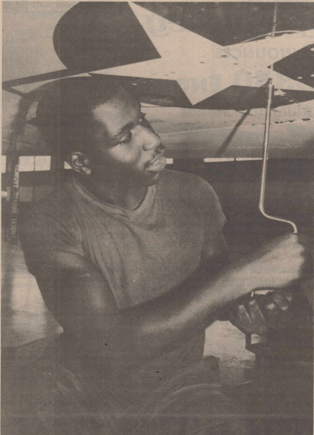
AIC James Lee assembles the panels on a T-38 wing after a phase inspection, which was rated excellent by Quality Assurance. Airman Lee is assigned to the 64th Organizational Maintenance Squadron, Fox Dock. The native of Philadelphia, Pa. has been assigned to Reese for one and one-half years.
