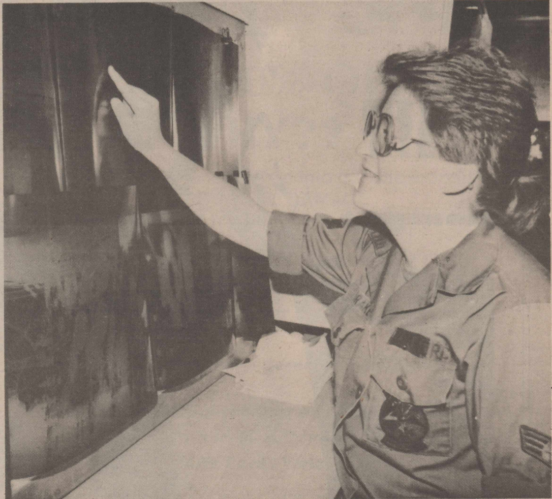
Senior Airman Susan Drake inspects the x-rays of various aircraft pieces. This is the second step of the x-ray process done on many aircraft parts.
