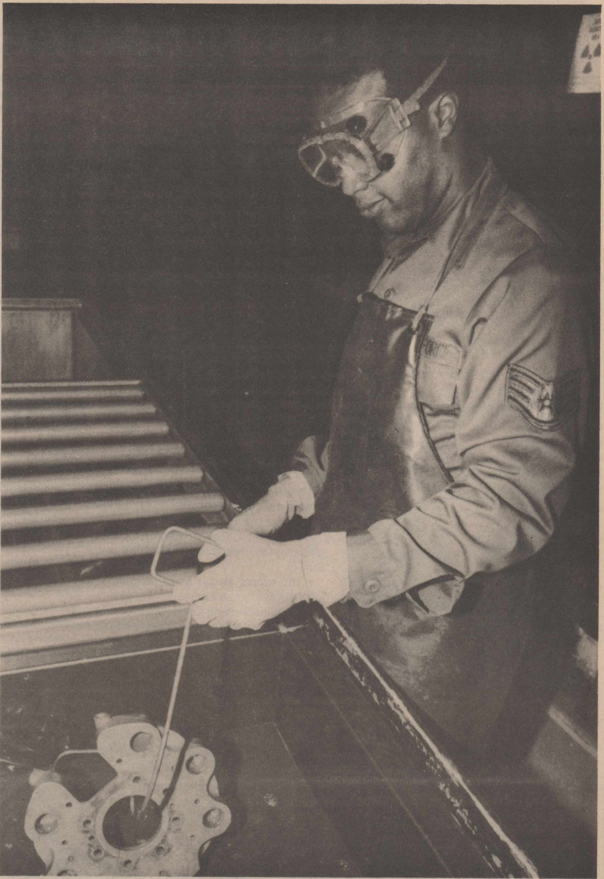
Staff Sergeant Antonio Buchanan dips a brake housing in penetrant while checking for defects. This is the first step of the inspection process.
