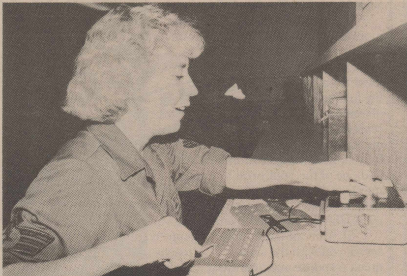
Sergeant Valorie Riffle uses an eddycurrent unit, which sends an electromagnetic field which checks for surface and near surface cracks.
