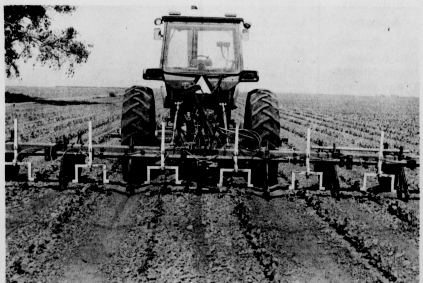
H-E-C SPRAYING RIG attached to a tractor which was being used to spray weeds in a cotton field just north of Abernathy. The H-E-C sprayer can effectively kill weeds at a speed of four miles per hour. It saves the farmer chemical, time and labor.
