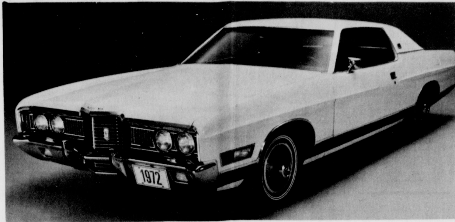
A fresh front-end treatment highlighted by a new grille marks the 1972 Ford LTD. Composed of a one-piece center section flanked by separate outer sections, the grille emphasizes the long elegant look of the 1972 Fords. The new front bumper is designed with a center bar to protect the grille.
